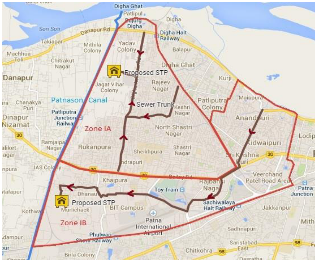
Figure 6-1: Suggestive alignment of sewer trunk in Zone IA and Zone IB (Digha)
