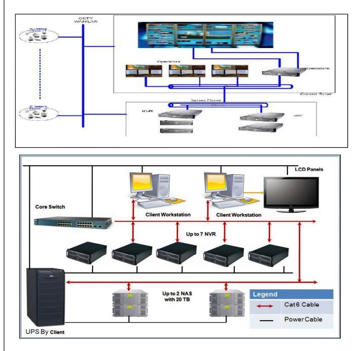
The main servers and video management application will be placed at Main Control Room with a Core Switch connecting the main camera Network from sub-Control room to the Main server at Central Control Room. The Monitoring stations are connected to the network via switch and will be places at various stated viewing locations across the cities. The Viewing station will be directly/indirectly connected to the main server for retrieving the recording or viewing the live video.
