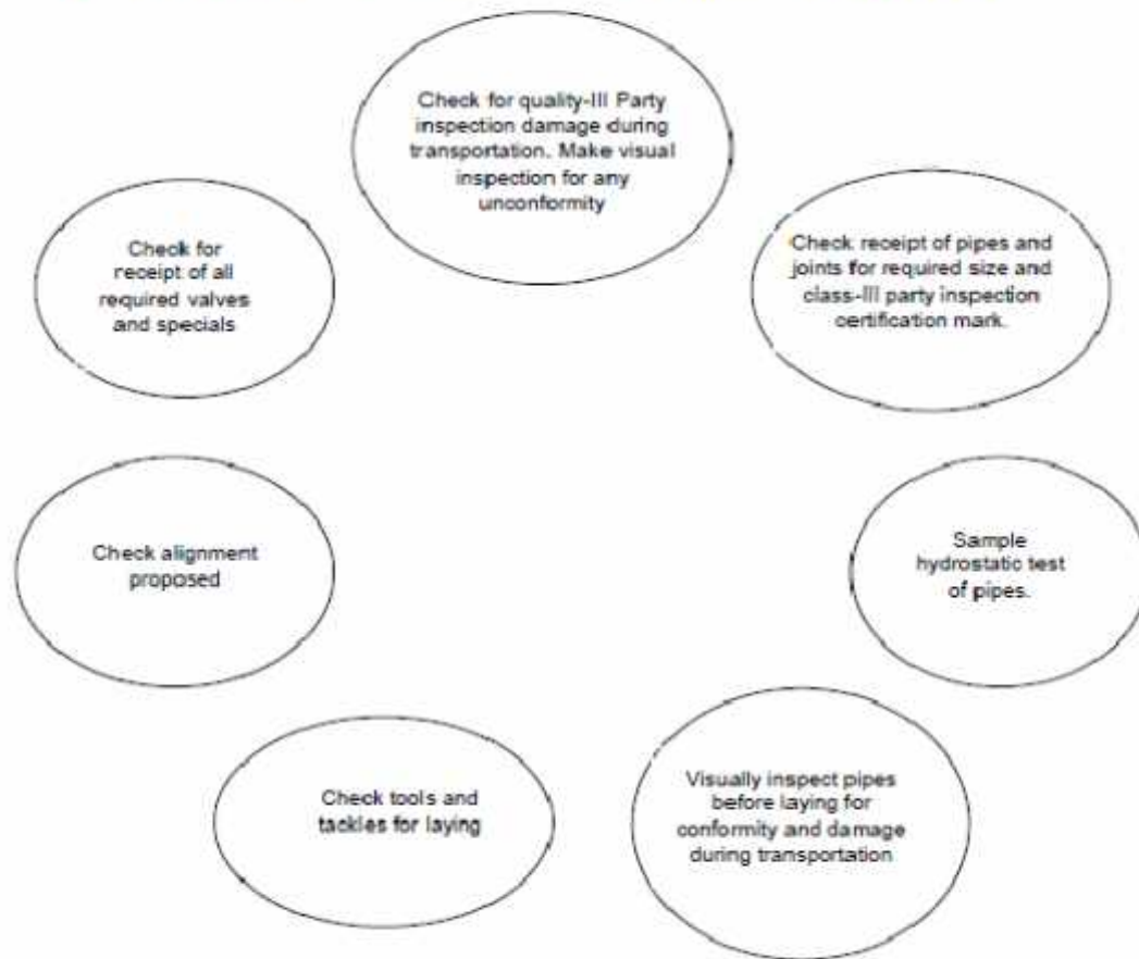
Figure 8.1 (b) CHECKS FOR PREPARATION WORKS BEFORE LAYING WATER SUPPLY PIPE LINES
